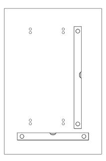
3. Using the drill and 8mm drill bit, drill into the marked positions then insert the wall plugs and tap flush to the finished wall surface.
