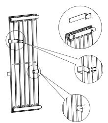
2. Set the position of the wall hanging brackets (on the wall) in relation to the size of your radiator, the brackets should be located between the last bar and the second bar in, as shown. Mark these positions on the wall in the required location and use a spirit level to ensure that these are horizontally and vertically aligned.
