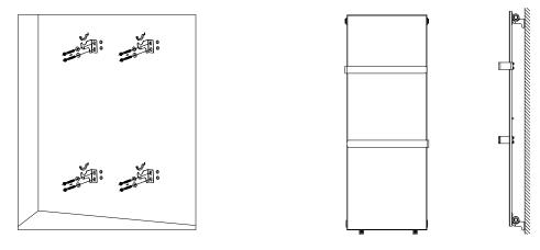
5. Once all brackets are secure, hang the radiator until fixed firmly into place and adjust so that the radiator aligns with the pipework.
